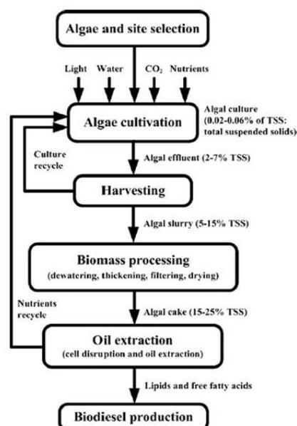
**Figure 4:** Process of biodiesel production in microalgae
