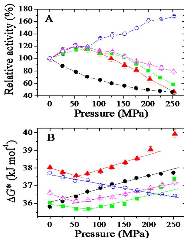
**Figure 9:** Pressure dependence of the relative activity (A) and activation free energy (B) of deep-sea DHFRs. Three deep-sea DHFRs—mpDHFR (red filled triangles), svDHFR (magenta open triangles), and sb21DHFR (green filled squares)—are compared with wild-type ecDHFR (black filled circles) and its D27E mutant (blue open circles). The experimental temperature was 25.0°C. Lines in panel B indicate linear fits. (Reproduced from Ohmae et al. [40].)
