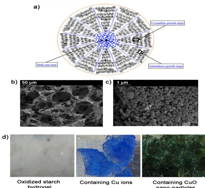
**Figure 5: Inner Starch Structure:** (a) Stylized model representing the distribution of amylose and amylopectin molecules. The blue lines represent amylose molecules, and the black lines represent amylopectin molecules [149]. FE-SEM images of (b) freeze-drying starch-siloxane scaffold, and (c) mineralized hydroxyapatite on the scaffolds [148]. (d) Photography's of oxidized starch hydrogels [151]. Copper ion (Cu) and copper oxide (CuO) nano-particles were incorporated into the hydrogel matrix.
