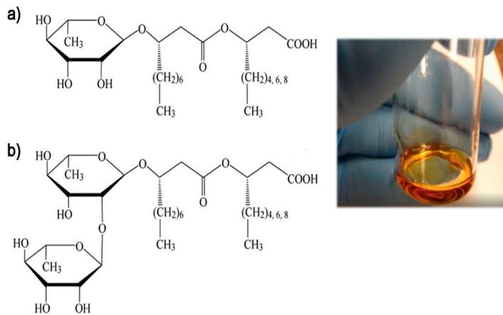
**Figure 6:** Structure of Rhamnolipids: Under typical growth conditions with *Pseudomonas aeruginosa*, two main rhamnolipids homologues are obtained: (a) monorhamnolipid (RL-1) and (b) dirhamnolipid (RL-2) [157]. Image of Rhamnolipids extract [3].
